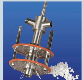
**Packed-bed impeller** optimizes yields of secreted products; basket is filled with Fibra-Cel® disks and used with a patented low shear draft tube impeller
