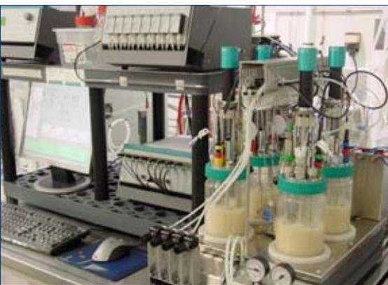
Figure 1. DASGIP system for biomass and protein optimisation and reaction engineering.
