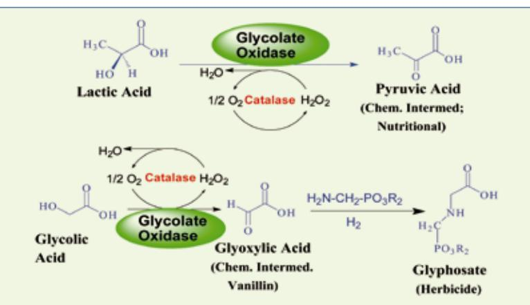
Figure 2. Glycolate oxidase (GO) now serves as a one enzyme one optimised process and several products platform. The process platform has been patented.
